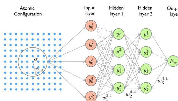
A dropout NN potential with two hidden layers (dashed arrows indicate dropped connections)
