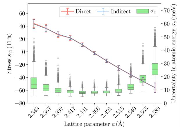
Potential part of the 11 component of the virial stress in a monolayer graphene (red and blue error bar plot), and uncertainty in atomic energy (green box plot) at various lattice parameters
